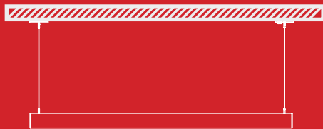
SUSPENDED (with aircraft cables)
